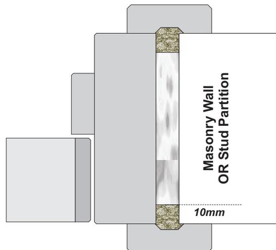
For installation gaps 10 ~ 15mm the gap between the back of the frame and the surrounding structure must be tightly packed with mineral fibre between fixing positions.
