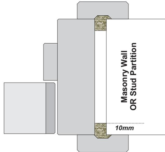
For installation gaps up to 10mm where other details do not satisfy Fig. 14.7 requirements the gaps must be sealed on both sides of the frame with an acrylic intumescent mastic to a minimum depth of 10mm.
