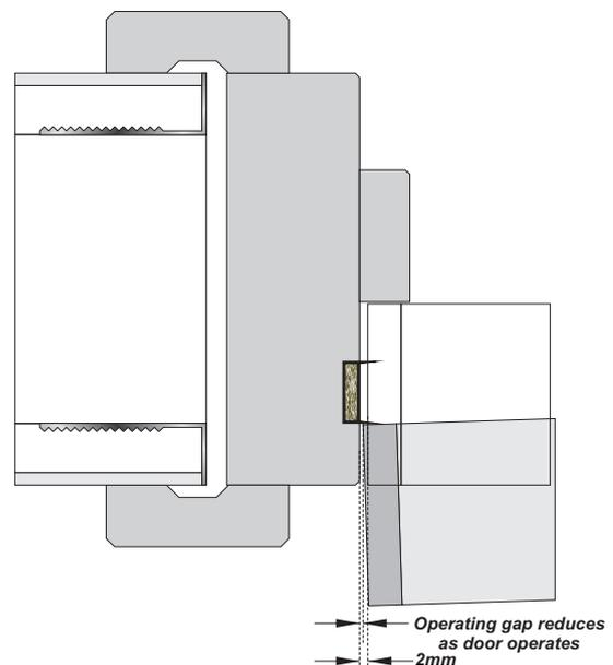
**If door leaves are fitted with square edges and corners when used with doorsets fitted with combined intumescent / smoke seals the following difficulties may be experienced:**
