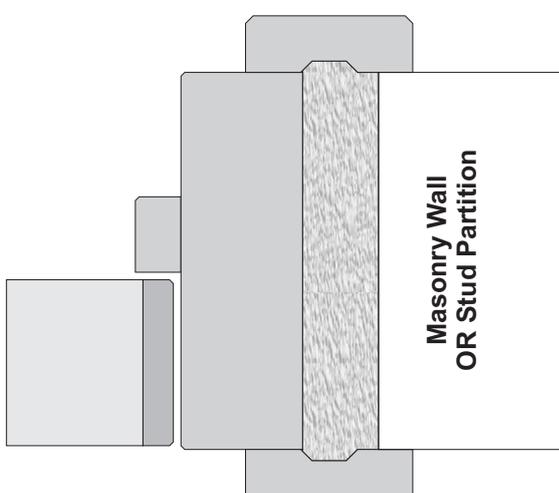
**Installation gaps in excess of 20mm are not approved and the opening must be adjusted by the use of timber grounds or in other ways to create prepared openings.**
