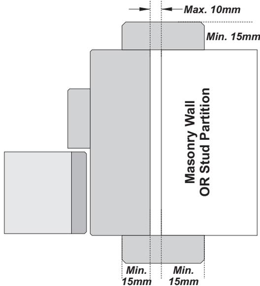
For timber stud partitions and masonry walls built without fair face, fire rated doorsets may be fitted to prepared openings without the use of additional intumescent materials where the gap between the frame and the surrounding structure is less than 10mm and where architrave, that is not less than 15mm thickness, overlaps the frame and the surrounding structure by not less than 15mm.
