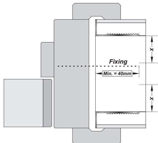
**a/ Steel fixings to penetrate structure to a minimum depth of 40mm.**
